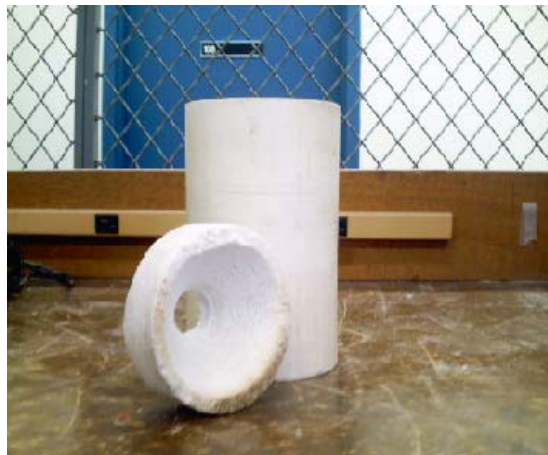
Figure 4.2.8c Machined ceramic material used to smooth the transitions of the fluid in the pipe.
